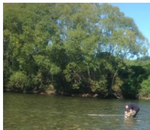
Fraser Lucas testing at Alexander Bluff Bridge (25 Feb) - black disc water clarity 5.4 metres, temp 17°C.
